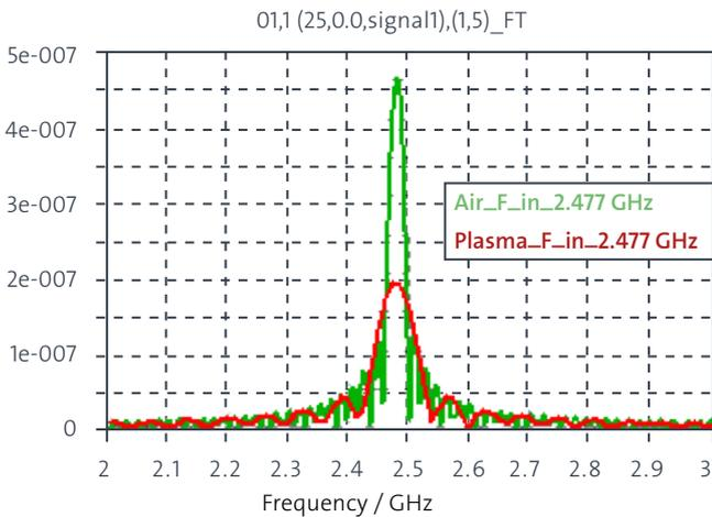
Figure 5: Output signal from Fourier Transform, showing the effect of ionization on the resonance.
