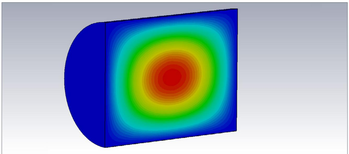
Figure 4: TE111 mode with Eigenmode solver.
