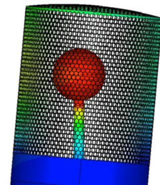
Figure 11: Temperature profile of misaligned mesh (5° rotation respect to horizontal axis).
