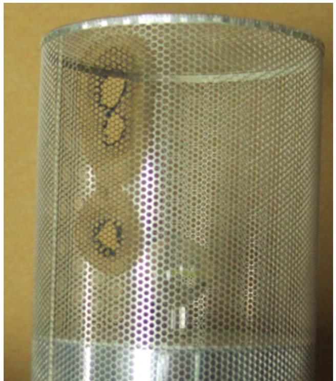
Figure 14: Hole on a mesh caused by misalignment.
