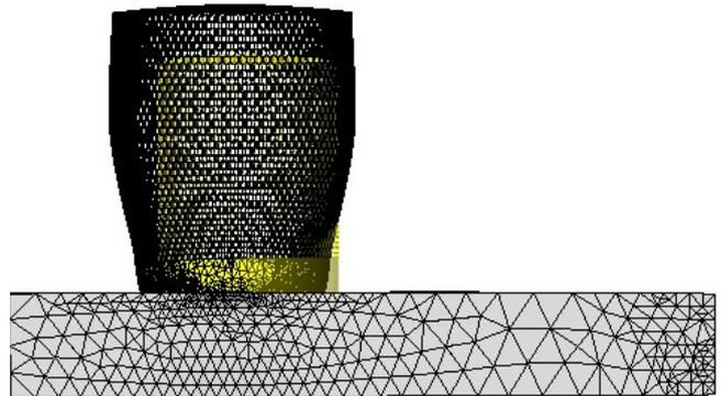
Figure 12: Exaggerated deformation from mechanical simulation.
