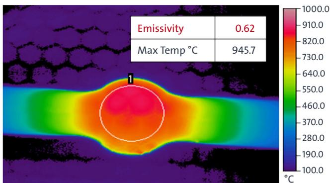
Figure 2: Temperature measurement profile.
