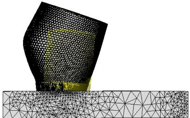
Figure 13: Exaggerated deformation of misaligned structure.
